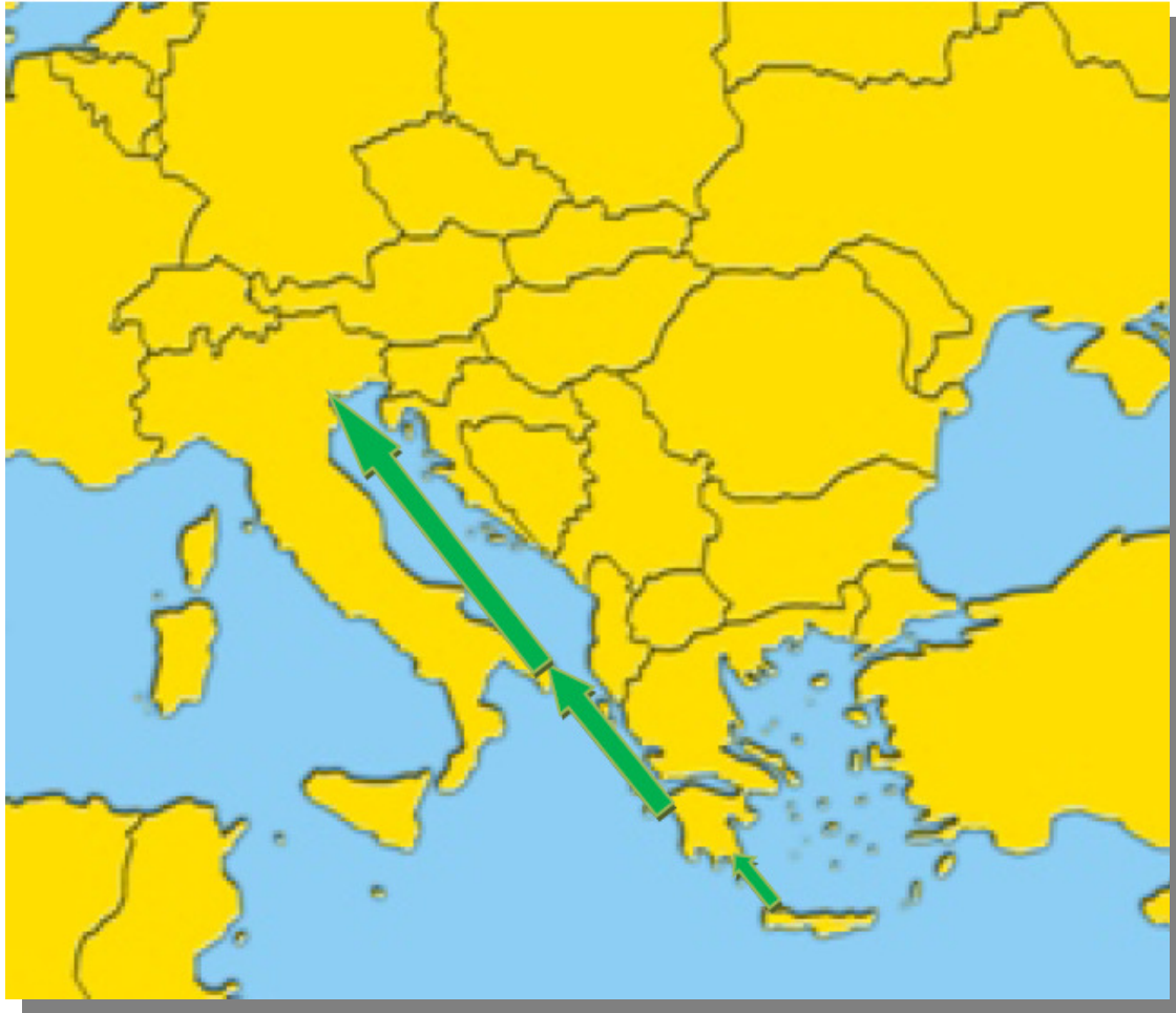
Fig. 6: The proposed interconnection of south Greece to north Italy by submarine cables based on HVDC technology and then to the electricity markets of the central European countries - Interconnection of Crete to Southern Peloponnesus
